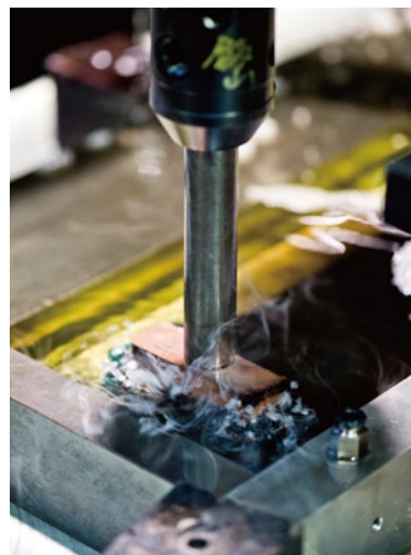
Sinker EDM in operation. The secret to highly accurate machining is electrodes, jigs and tools developed in-house.
