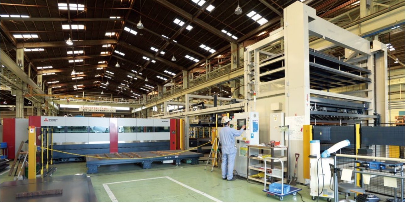
The laser processing system installed this time. The ML4020RX is shown to the left as sheet metal is automatically carried to the work area from the storage racks using the special-purpose feeder.
