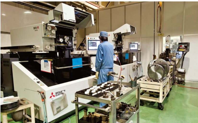
MV Series – The wire-cut EDM made by Mitsubishi Electric installed in the fall of 2015.
