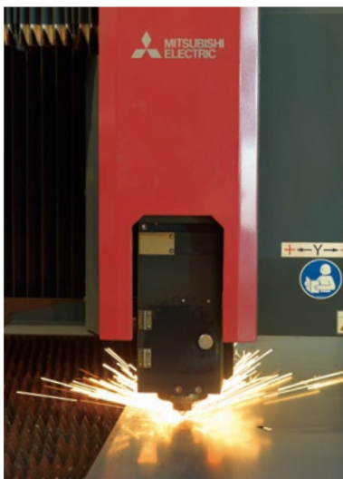
The laser processing machine installed has an output of 4.5kW and can cut sheet metal up to 25mm thick.
