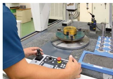
Final CMM measurement inspection of a cold-forging die manufactured in an EDM.
