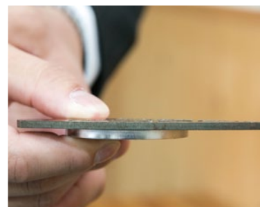
Stainless steel with a top section processed in oxygen and bottom section processed in nitrogen. The difference between cross-sections is clear.
