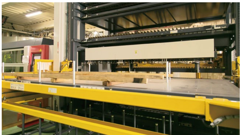
When Ueno Tekko installed the eX-F60, it also installed the 30SCX-eX-F, a stocker capable of high-speed sheet changing. This significantly improved work efficiency as material can be automatically loaded into the machine.
