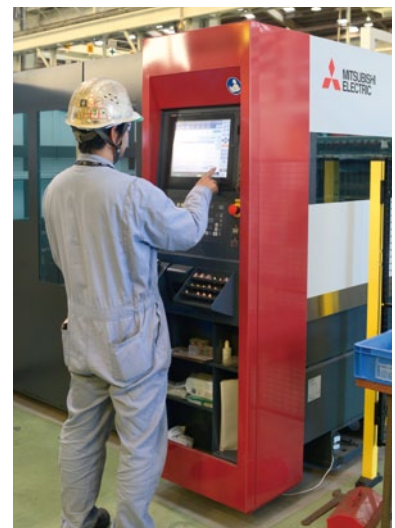
CNC unit of the laser processing machine. Customers report that data can be loaded with greater ease than previously possible.
