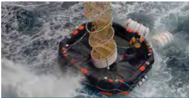
Liferafts are lowered with the chute
