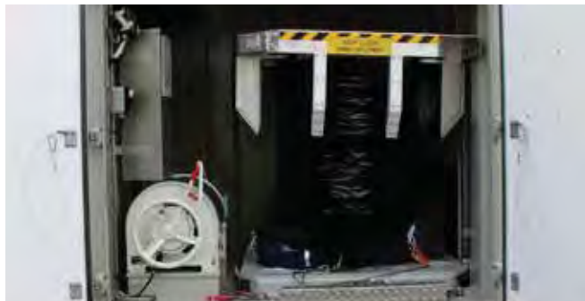
Launching begins. Liferafts are lowered with the chute
