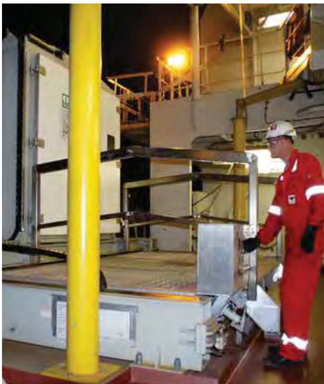
A hydraulic slide moves the evacuation system into cantilevered position for deployment.
