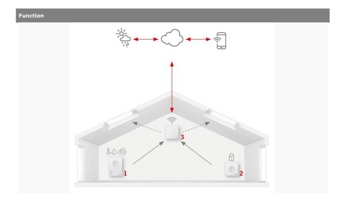
The VELUX ACTIVE gateway (3) is the 'heart' of the VELUX ACTIVE system. It is connected to both the local WiFi router (internet), to the io-homecontrol<sup>®</sup> VELUX INTEGRA<sup>®</sup> products, to the indoor climate sensor (1) and to the departure switch (2). When VELUX ACTIVE is installed, operation of VELUX INTEGRA<sup>®</sup> products can be performed in 4 different ways in addition to using VELUX INTEGRA<sup>®</sup> remote controls:
