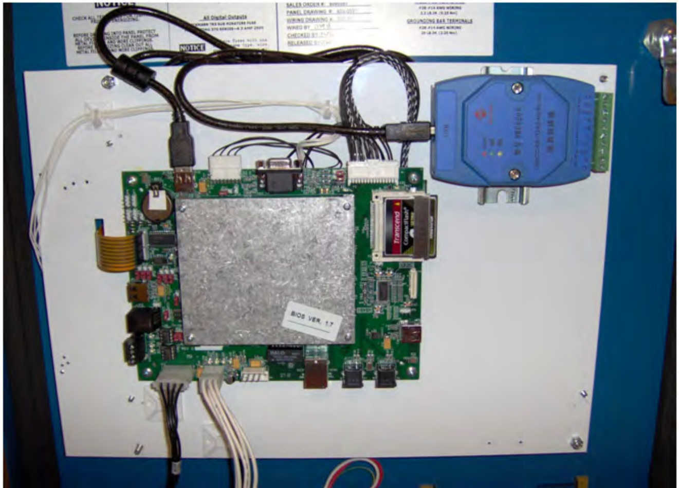
Figure C-2. Vission 20/20 Single Board Computer with USB to RS422/RS485 Converter (VPN3485C) on USB port P18
