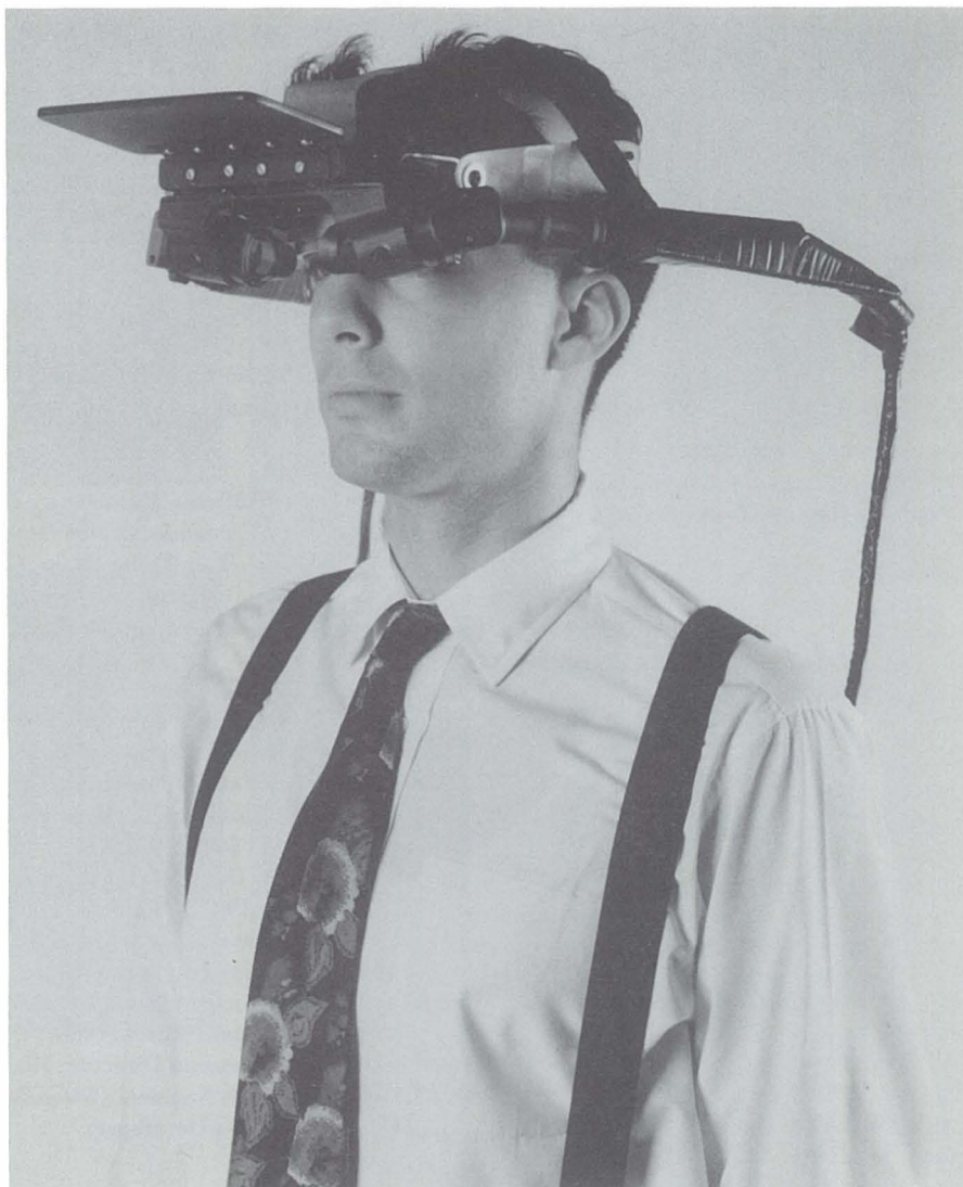
"The fundamental idea behind the three-dimensional display is to present the user with a perspective image which changes as he moves," Ivan Sutherland wrote. "The image presented by the three-dimensional display must change in exactly the way that the image of a real object would change for similar motions of the user's head."
