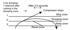
When a "stop current" continues for 2.5 seconds after rushing on the stop zone, the compressor operation stops.
