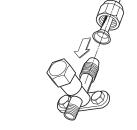
Finally, tighten the flare nut with torque wrench until the wrench clicks.
