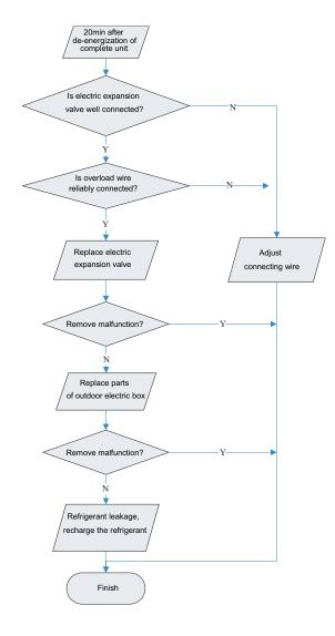
(7) Process of outdoor unit communication circuit detection
