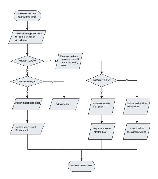
(2) Indoor fan does not rotate without feedback
