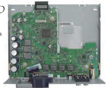
Large Capacitor and Plate-Type Heatsink
