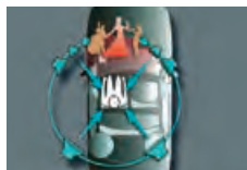
Time Alignment Image Digital delay processing makes all speakers sound as if they are virtually equidistant from the listener, for a clearer, front-focused soundstage.
