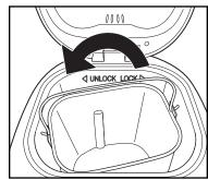
Using the bread pan handle, turn the bread pan counterclockwise to unlock it. Lift up and remove bread pan from baking chamber.
