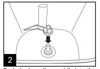
Push the kneading paddle into the drive shaft inside the bread pan. **CAUTION!** Falling Object Hazard. Breadmaker can wobble and walk during kneading cycle. Always position it in the center of the counter away from the edge.
