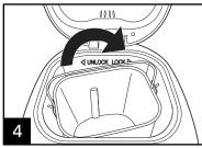
Place the bread pan into the appliance and make sure it is firmly locked in place by turning it clockwise. Close the lid.
