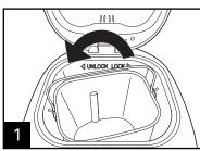
Using the bread pan handle, turn the bread pan counterclockwise and then pull it out of the appliance.
