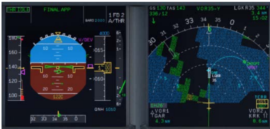
Picture 110: Manual Approach after passing MDA (ND = ARC mode)
