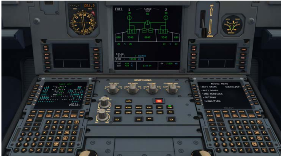
Picture 3: ECAM and Upper Pedestal view, selected with [F10]
