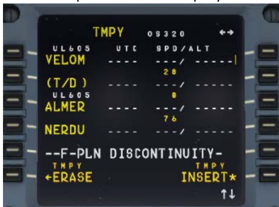
Picture 132: Temporary flight plan after enabling ALTN
