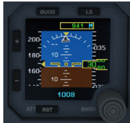
Integrated Standby Instruments System (ISIS)
