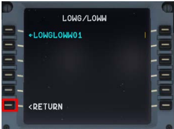
Picture 136: Not using existing CO RTE
