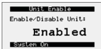
The unit ships from the factory in a disabled state. To allow the unit to operate, the controller must receive a run command from digital input U4. **Jumper unit terminals R - G to allow the unit to operate.**
