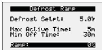
This screen only appears if the unit has an energy recovery wheel and a frost control method was provided with the unit.
