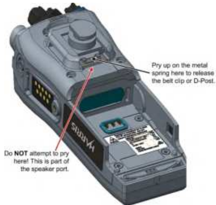
Figure 4-3: Remove Belt Clip
