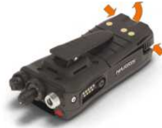
Figure 4-2: Remove the Battery
