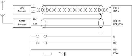
**NOTE:** The field power supply *(see page 66)* connected to UB+ and 0 VDC pins is an auxiliary power supply (different from the main power supply).
