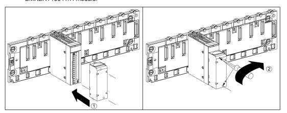
The following table describes the assembly procedure of the 28-pin terminal block onto a BMXERT1604T/H module:
