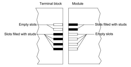
The following diagram shows an example of coding configuration with which it is not possible to fit the terminal block to the module.
