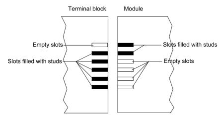
**NOTE:** The module connector has indicators which show the proper direction to use for terminal block installation.
