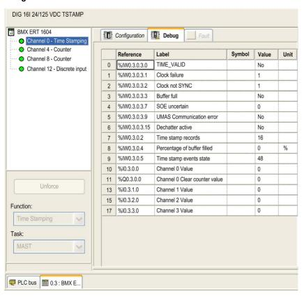
The parameters for the group 0 (channels 0...3) debug page are listed in the following table. Group 0 inputs are dedicated time stamping inputs, which cannot be reconfigured as counter or standard discrete input channels.
