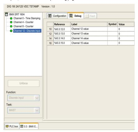
The standard discrete input (without time stamping) parameters for the group 1, 2, 3 debug page are listed in the following table:
