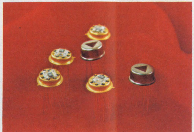
High accuracy op amps with FET inputs, the Analog Devices AD506, have a maximum offset of 0.1 mV, 10\mu\text{V}/^\circ\text{C} , maximum drift and 5-pA maximum bias current.
