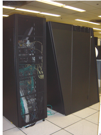
Argonne's 5.7 teraflops system (BGL) 1024 nodes, 2048 processors, 512 Gbytes RAM www.bgl.mcs.anl.gov
