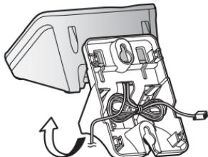
5 Mount the unit on a wall then slide down to secure in place.
