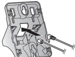
2 Tuck the telephone line cord inside the wall mounting adaptor (1). Connect the AC adaptor cord and telephone line cord (2).
