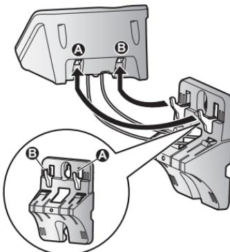
4 Adjust the adaptor to hold the base unit, then push it in the direction of the arrow until it clicks into place.
