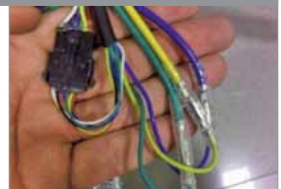
Locate and disconnect the cables that connect the controller to the MOTOR (BLUE, GREEN and YELLOW cables and 6 pin plug).
