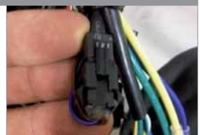
Locate and disconnect the cables that connect the controller to the TORQUE SENSOR (3 pin plug).
