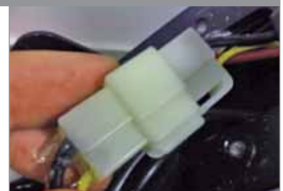
Locate and disconnect the plug that connects the controller to the BATTERY (white plug).
