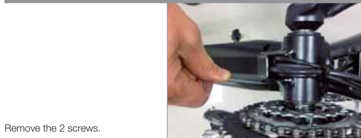
Locate the 2 screws located in the down side of the frame, next to the bottom bracket.
