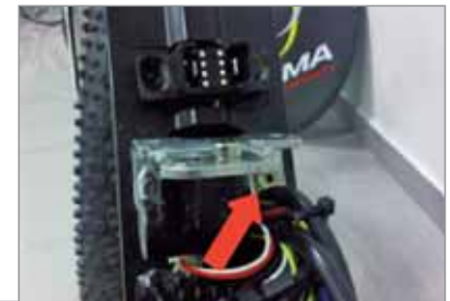
Locate and remove the 2 screws that fix the battery lock plate.
