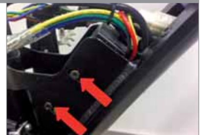
Locate and remove the 2 screws that fix the controller to the frame reinforcement plates.
