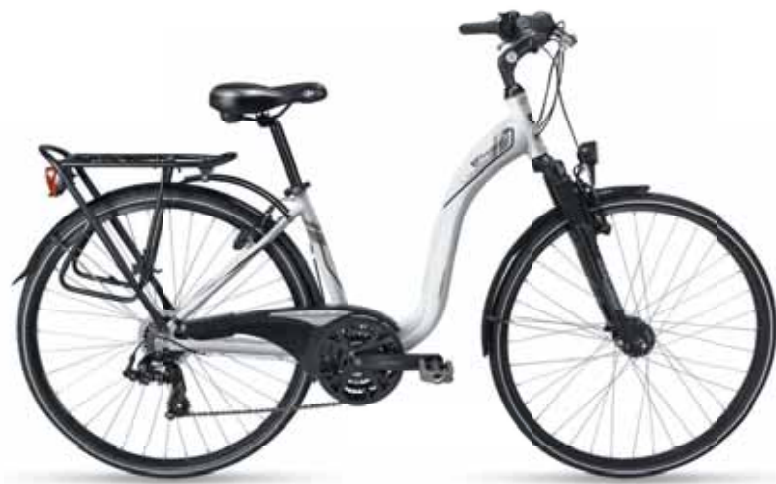
London wave TE663 Alloy Hydrof. 28" City Wave Suntour XR-178 3 SP SM, MD, LA Suntour M-3010 Rubena 700*35 16,8 Shimano TX55 7 SP Shimano Dinamo
