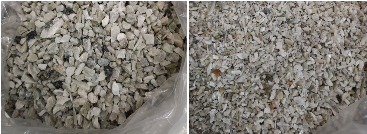
Figure 19 - Coarse and fine DMS concentrates produced from Piedmont composite samples
