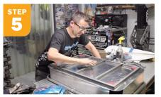
Cut 3/4" steel tubing to create the steel support frame with three cross beams for under the bed of the wagon. Tack weld everything in place, then weld together.
