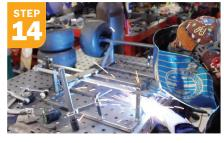
Locate and weld front spindles to match the rear axle height center line so the wagon will ride level and clear the bed when turning.
