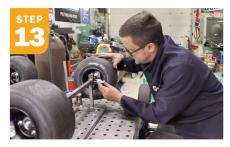
Use a piece of poster board to create a template for the brackets, then cut out two brackets using your steel plate. Sand down with a belt sander and drill a hole at the top. Weld the brackets to spindles for steering.
