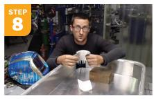
Use a piece of poster board to create a template for the four corner pieces, then cut out and bend each using a slip roller. Tack weld each piece into place before fully welding them in.
