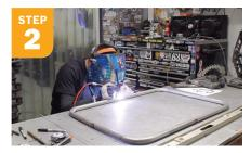
Bend 1" aluminum tubing to the desired shape and tack weld the pieces together to create the outer edge of your wagon.
