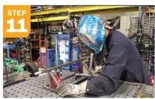
Cut and MIG weld four pieces of steel tubing (two vertical, two diagonal) to the rear axle and steel frame. This will support and hold the axle in place at the correct ride height.
