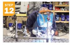
Fabricate and TIG weld two steering knuckles with 1/4" thick, 1" wide steel plate. Note: The knuckles should fit inside the rim without touching. Once complete, MIG weld them to each side of a piece of box tubing, which will be your front axle. Then, MIG weld two pieces of box tubing to connect the front axle and steel frame, similar to Step 11.
