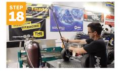
To finish, fabricate the handle and front clip. Weld the handle to the steel frame and the front clip to the front of the wagon, which will hold the handle in place. The handle should clear the bottom of the wagon and be straight up when not in use.
