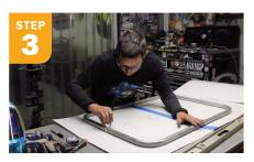
Trace the inside of your aluminum tubing onto a piece of poster board to create a template for the bed of the wagon. Then, using your template, cut the aluminum sheet metal to size with your pneumatic sheet metal shears. Be sure to include extra material for each of the four sides of the wagon. This design included 6" on each side. Once everything is cut out, bend each side at a 90° angle with a stomp shear.
