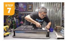
Next, line up the steel frame with the bed of the wagon and drill five countersunk holes to align with the mounting tabs added in Step 6. By countersinking the holes, the bolts will sit flush on the bed of the wagon instead of sticking out. Use bolts to secure into place. This design used 3/4" bolts with nylon lock nuts and countersunk washers.
