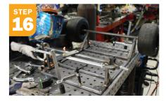
Fabricate diagonal struts to support the steering axle and clearing the wheels when turned.
