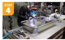
Fit the aluminum sheet snug to the aluminum tubing and tack weld together.
