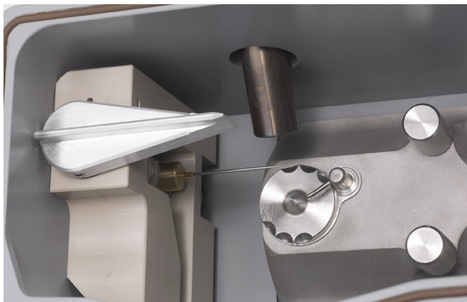
Figure 33. View of the corona pin in the operational position for the APCI mode
