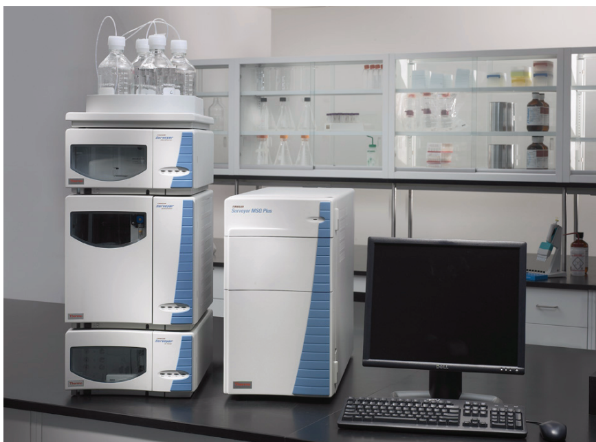
Figure 1. View of the Surveyor MSQ Plus MS detector and the Surveyor LC system
