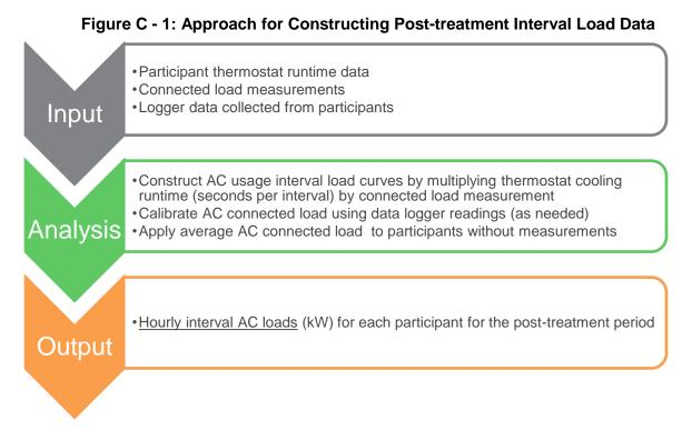
Note that loads were calibrated by taking max average proxy day load for corresponding logger and runtime data and applying to runtime. This adjustment was based on the observed difference between spot load measurements and logger measurements. This was done to help get loads closest to what they should be on proxy and event days during event hours.
