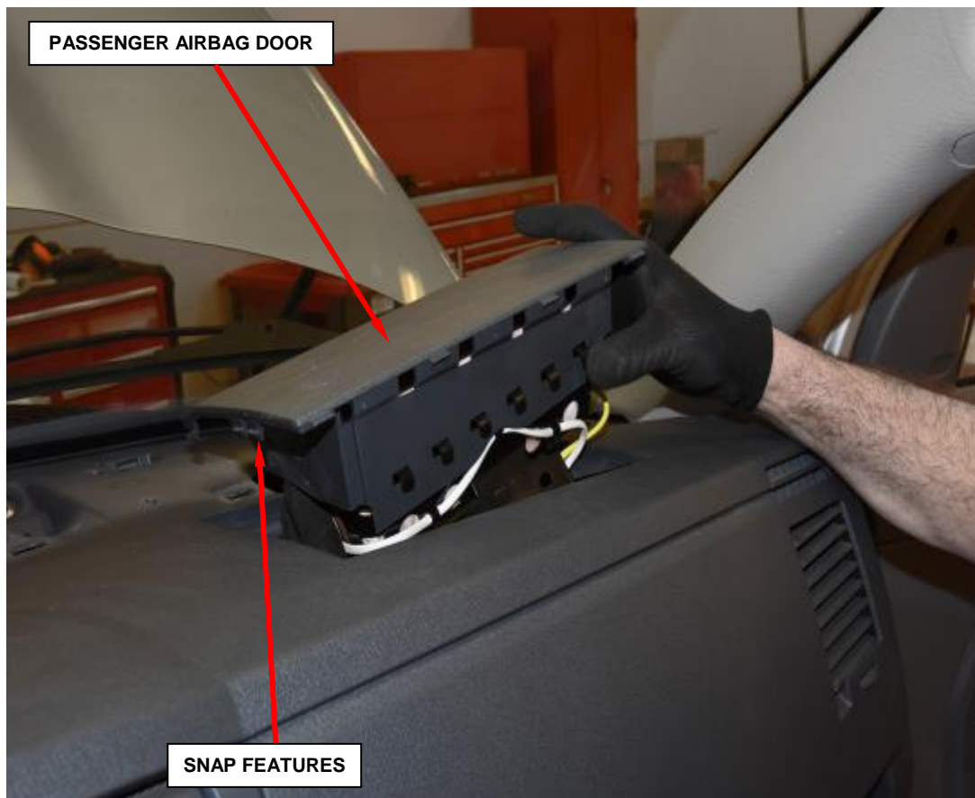
Figure 31 – Passenger Airbag Removal
