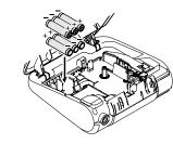
Insert a tape cassette, making sure that it snaps into place. End of tape
