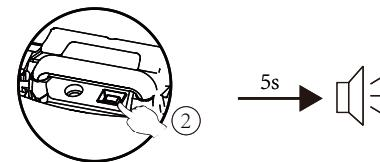
Press and hold WIFI button on mower console pad and then switch on the main power of mower.
