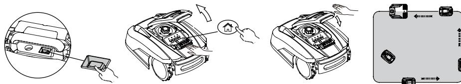
Once the device has docked, the symbol will start flashing. This indicates that the battery is charging correctly.
