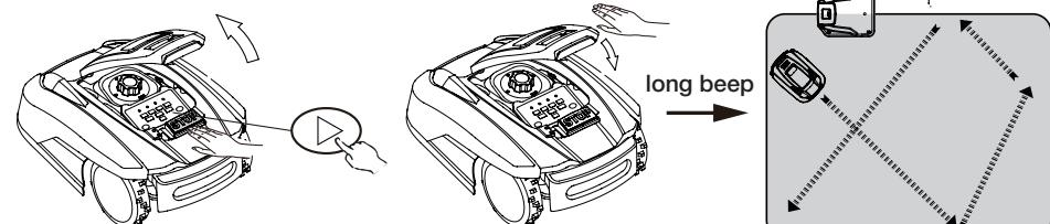
Press start button and close the top cover, Robotic Mower will start to work after you hear a long beep.
