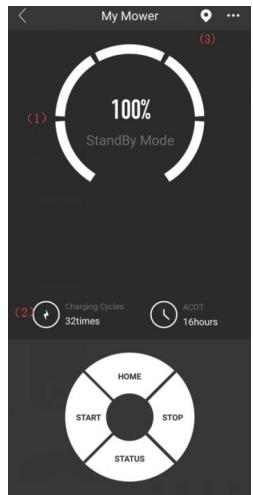
This is our mower main control interface, you will battery volume and working mode from upper graphic and remote console pad from lower side.
