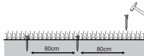
When first planting the pegs, do not drive them fully into the ground. Use a light hammer to drive them in a little bit. Also locate the fixing pegs and lay each one on the lawn at approximately the correct distance from lawn edges (20-30cm) and obstacles.
