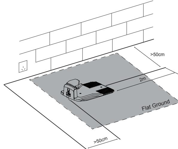
Do not place the docking station too close to a slope, such as at the top of a hill or the bottom of a furrow. Avoid left and right inclination in excess of 5 degrees.
