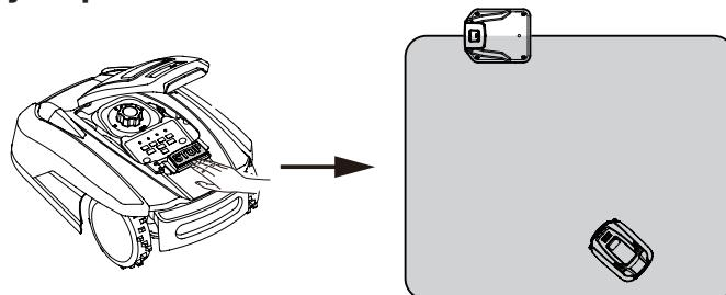
Press **STOP** button to break the mower at any time.
