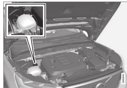
Coolant expansion tank.
