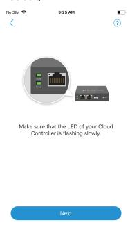
4) Click **Next**. To bind the Omada Cloud Controller to your TP-Link ID, you can either scan the QR Code, or enter the device key manually. The QR Code and device key are displayed on the back of the Omada Cloud Controller.
