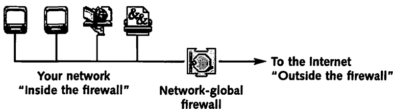
Figure 17.20 Machines inside the firewall provide a significant additional security risk if they are compromised.
