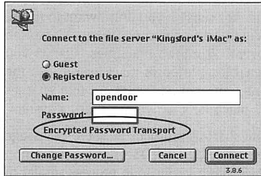
Figure 14.7 iDisk and Mac OS X servers use an alternative AFP login process called DHX. Like AFP's standard login process, DHX is much more secure than FTP.
