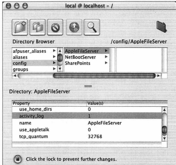
Figure 18.22 Turning on the File Sharing log is one of the few tasks for which you should consider using NetInfo Manager.
