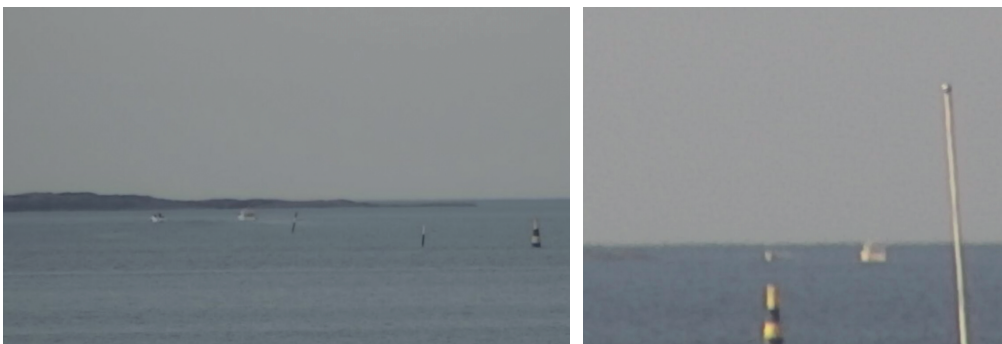
Figure 5: Picture on the left – two boats at 6.8 km (leftmost the “Small pleasure craft” and rightmost the “Medium pleasure craft”). Picture on the right – the same boats at approximately 9.6 km. Note that the zoom settings of the pictures are different.
