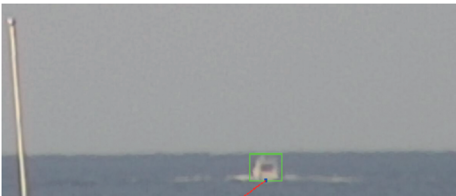
Figure 7: Deep neural network-based detection of the “Medium pleasure craft” at around 9.6 km.
