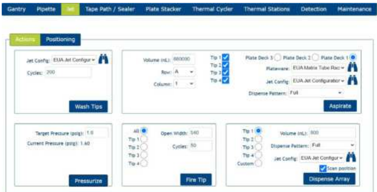
Figure 24. IntelliQube daily startup up routine operations control screen.
