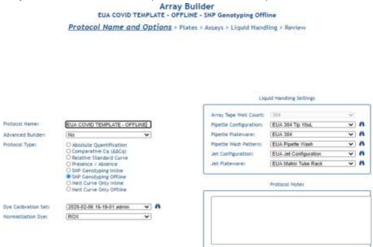
Figure 27. IntelliQube end-point protocol setup screen.
