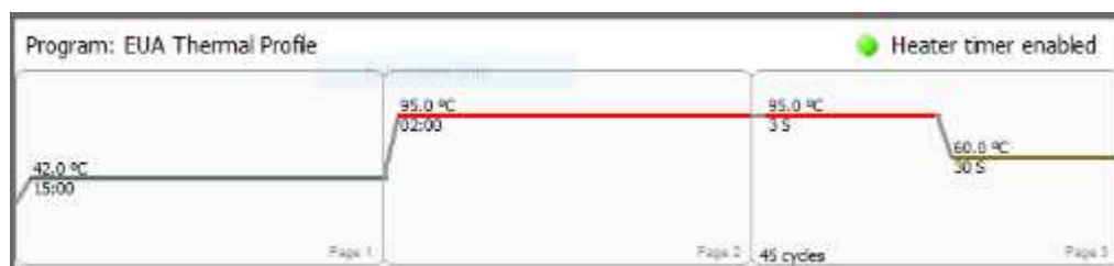
Figure 33. Thermal cycling parameters for the Hydrocycler 2 .
