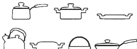
**For proper functioning, all pots and pans must have a plane magnetic bottom (a magnet must stick to it). We recommend pans/pots with a diameter between 12 and 24 cm for better results.**
