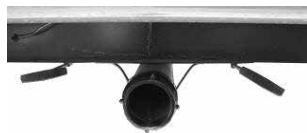
Black/Grey Tank Drain and Valves
