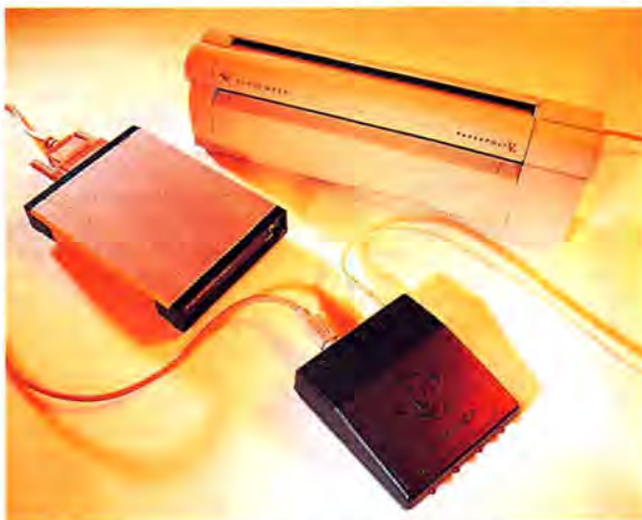
figure 2 / Get more serial ports by using Port Juggler. It costs more (about $100) than a plain-old serial-port switcher, but it comes with software to make switching among serial devices easier.
