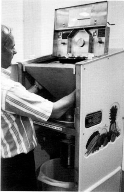
Figure 1c. Lifting out hopper
