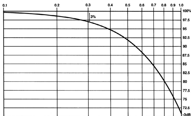
Figure 4.8. Bandwidth derating curve.
