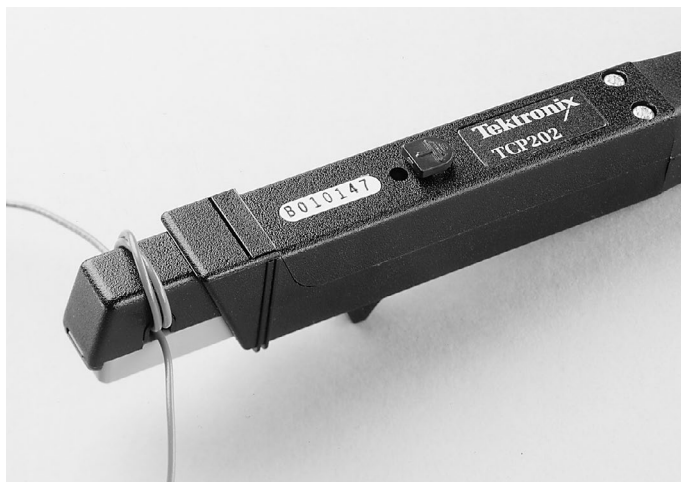
Figure 2.8. An example of a split core AC current probe. Looping n turns of the conductor through the probe increases effective sensitivity n times.
