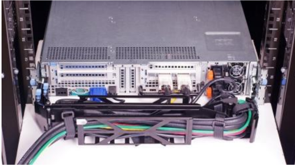
Figure 13. R815 CMA Mounted on the Side Opposite the Power Supplies (Recommended)
