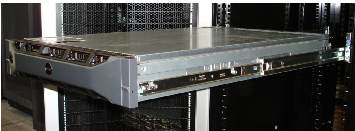
Figure 12. R815 Mounted in the B2 Sliding Rails
