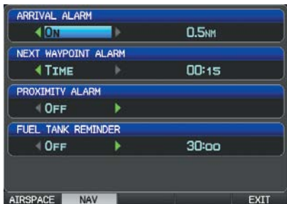
Nav Alarms (Split-Screen)
