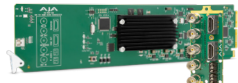
OG-ROI-SDI $1,045 openGear 3G-SDI to HDMI/3G-SDI Scan Converter with Region of Interest and Frame Synchronizer
