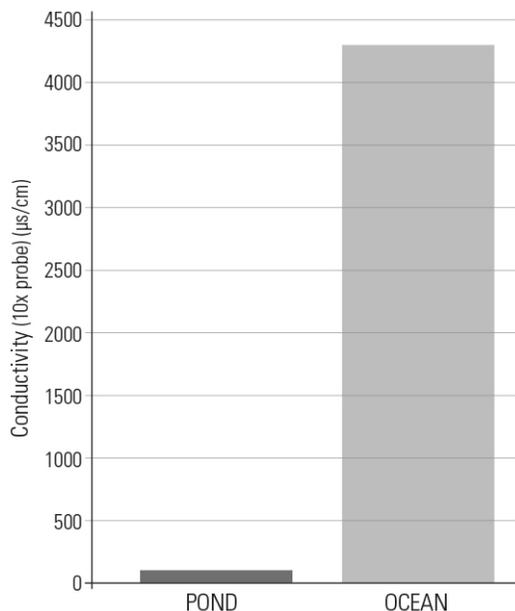
*Note: Original pond water and ocean water samples were diluted to 10% solutions to accommodate the conductivity sensor range.*
