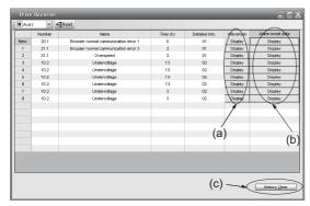
Click "Waveform" - "Display" ((a)) to display the graph preview window which shows data before and after alarm occurrence. For operating the graph preview window, refer to Help of MR Configurator2.
