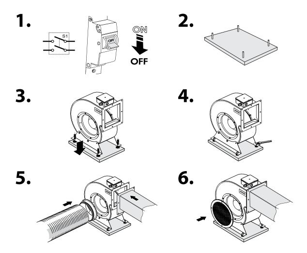
After installing the unit, you need to make sure that the fan impeller rotates freely.
