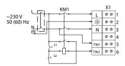
QF: automatic circuit breaker KM1: magnetic starter \$1,52: control buttons (QF, KM1, \$1,52 are not included in the delivery set) X1: terminal block
