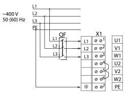
QF: automatic circuit breaker (not included in the delivery set) X1: terminal block
