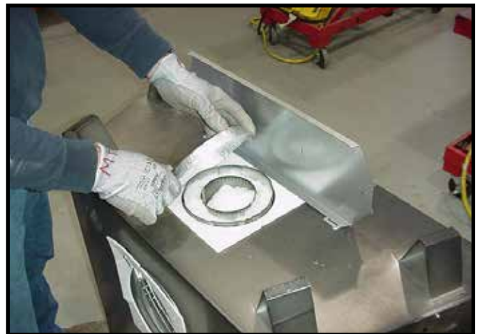
Figure 6.5 Remove the seal cap.
