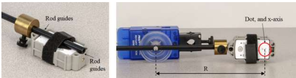
Figure 3: Attaching WAS to Pendulum Rod
