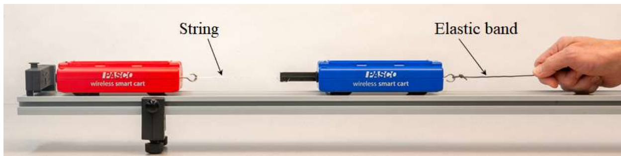
Figure 1: System Being Pulled By Elastic Band
