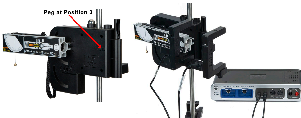
Figure 6: Measuring the Launch Speed
