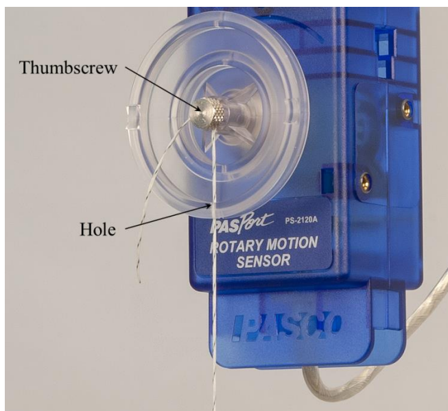
Figure 3: Attaching the string to the Rotary Motion Sensor
