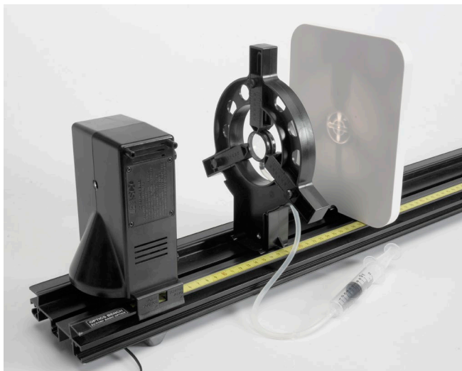
Figure 3: Adjustable Lens Setup
