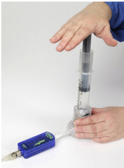
Figure 3: Compressing the Syringe
