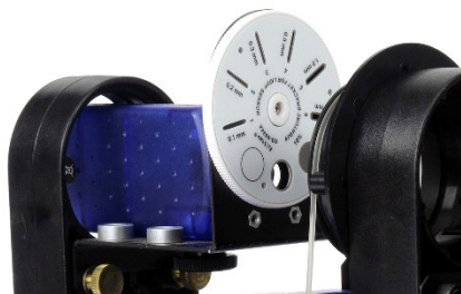
Figure 5: The Aperture Disk
