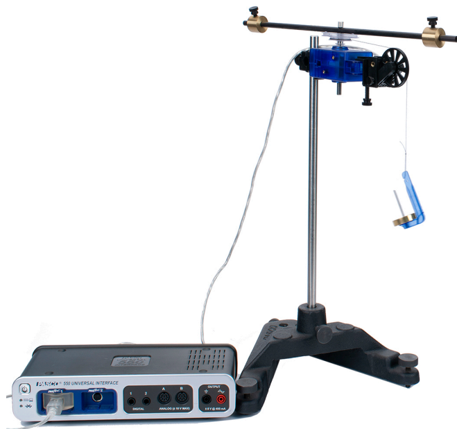
Figure 1: The hanging mass applies a torque to the shaft of the Rotary Motion Sensor and the resulting angular acceleration of the rod and brass masses is investigated.
