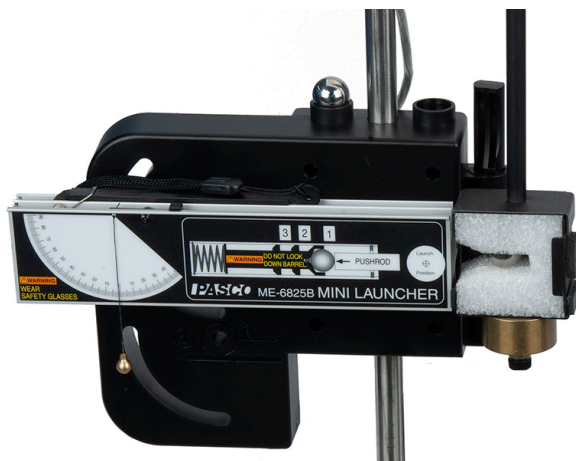
Figure 3: The pendulum must be adjusted so that the catcher is directly aligned with the launcher. When the ball is launched, it is trapped in the slot in the white foam.
