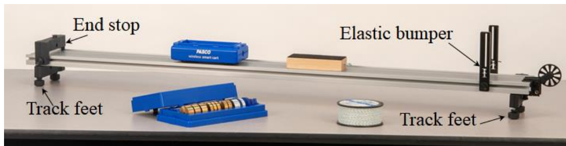
Figure 1: Setup for Newton's First Law
