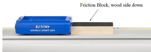
Figure 3: Smart Cart with Friction Block
