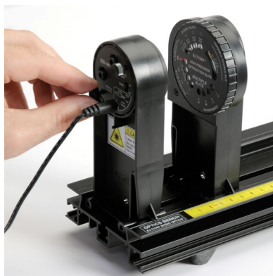
Figure 5: Aligning the Laser
