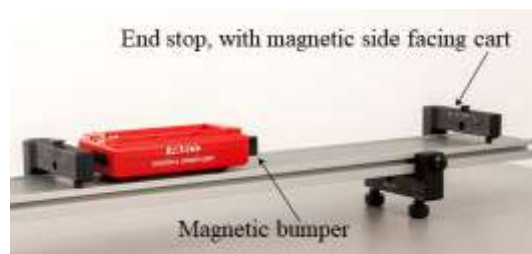
Figure 6: Cart with Magnetic Bumper
