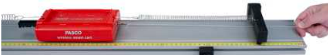
Figure 5: Pull on String to Determine the Spring Constant
