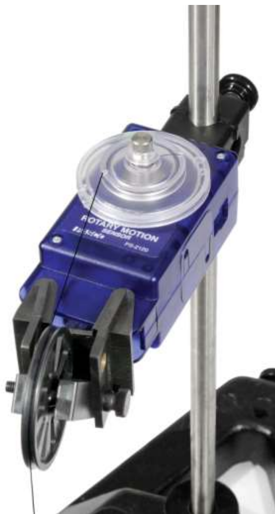
Figure 4: String and Pulley Setup
