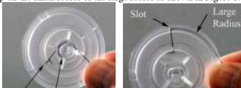
Figure 6: By running the thread through the slot, you can change the radius that the thread is wound around without having to re-tie the thread.
