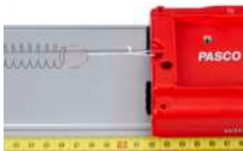
Figure 2: Attach Spring with Loop of String
