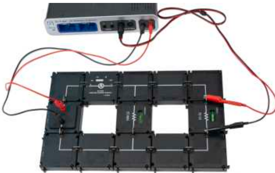
Figure 2: Parallel Resistors with Meters
