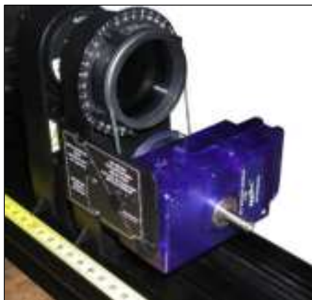
Figure 6: Rotary Motion Sensor Connected to Polarizer with Belt
