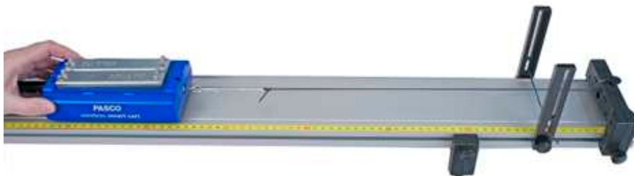
Figure 1: Setup with Elastic Cord Tied to Hole in Endstop
