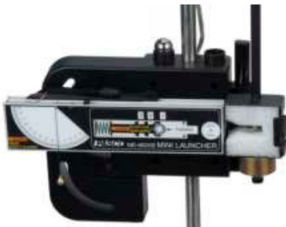
Figure 3: The pendulum must be adjusted so that the catcher is directly aligned with the launcher. When the ball is launched, it is trapped in the slot in the white foam.
