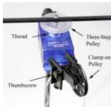
Figure 7: Adjusting Angle of Clamp-on Pulley
