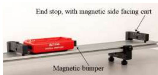
Figure 6: Cart with Magnetic Bumper
