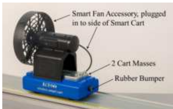
Figure 2: Cart with Bumper, Masses, and Fan
