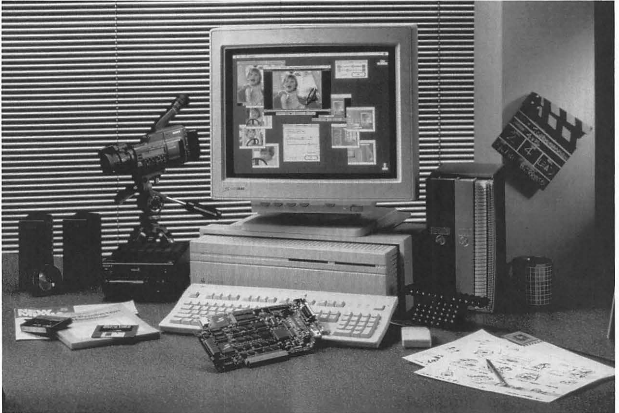
FIGURE 15.5: The VideoSpigot card and its output (photo courtesy of SuperMac Technology)
