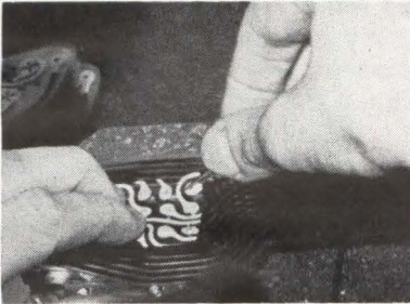
OPERATOR uses tweezers to press solder pads down over terminal pads
