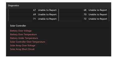
FIGURE 56: Solar Controller Diagnostics
