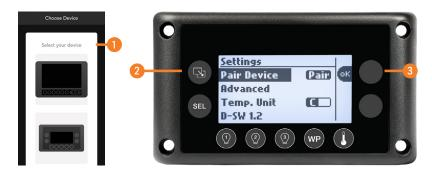
FIGURE 13: Pairing to the NODE
