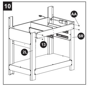
Secure the intermediate slide support (10) to the upper panel (13) by inserting screws (AA) through the slide support (10) and into the upper panel (13).
