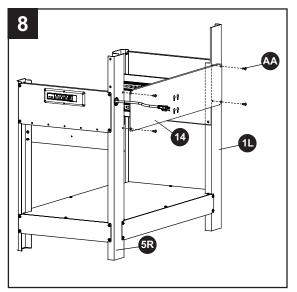
Loosely attach screws (AA) to the end of the intermediate slide support (10). Align the screws (AA) with the holes in the back panel (14), insert the screws (AA) into the holes and lower the intermediate slide support (10). Tighten the screws (AA).
