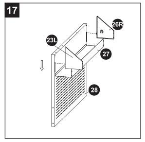
Secure the left and right storage cage side panels (23L and 26R) with screws (AA and BB).
