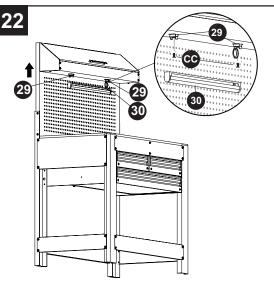
23. Install the light (30) into the light support brackets (29). Feed the light power cord (31) through the grommet in the pegboard (28). Plug the light power cord (31) into the light (30).
