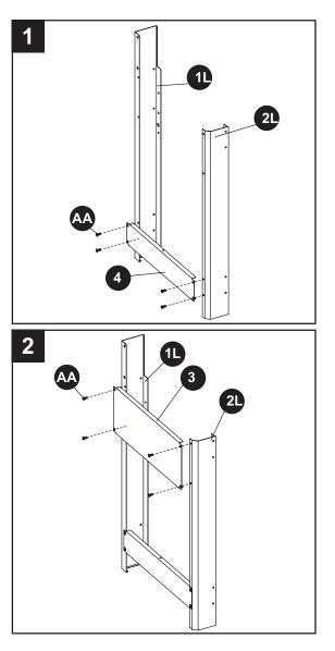
Attach the left side panel (3) using screws (AA). 2.
