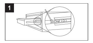
Pull the release lever up on the left side of the drawer. Holding both levers, pull the drawer out until the drawer releases from the drawer slides.
