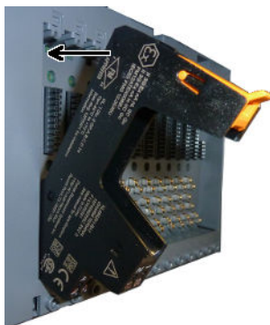
Figure 2-5: CHARM Terminal Block installation
