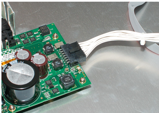
Figure 3-10: Disconnecting the Main board power cable from the Combiner board
