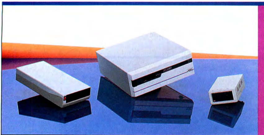
Last but Not Least (Left to right) Peripheral Land MacFast20, AST-4000, MagNet 20X. Peripheral Land's drive includes an intelligent tape drive controller. AST's drive stores 74 megabytes and includes a 60-megabyte tape drive. The MagNet 20X comes with InfoSphere's MacServe disk server software.
