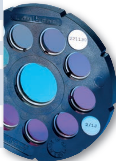
Test disc with colour-stable glass standards
